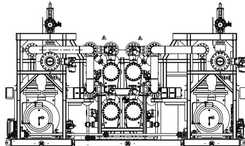
Self-priming, double entry, horizontal pump types
